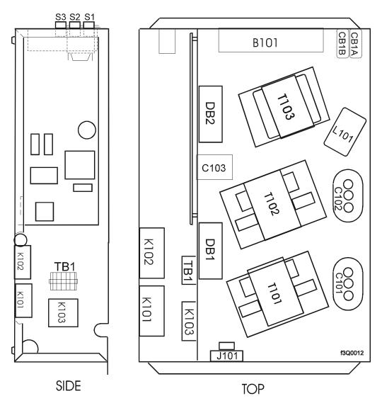
Figure 44. P300M/P300MQ Component Identification
